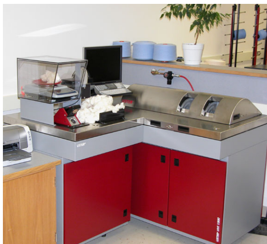
Figure 11. High Volume Instrument for testing cotton fiber
