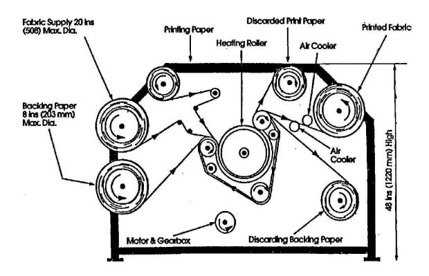
In general, fabrics printed using this technique must be treated with caution when being ironed or exposed to excessive heat. Also, these fabrics will exhibit all the other characteristics of pigment prints both good and bad. As a point of information, there have been a number of attempts to heat transfer reactive dyes employing a combination of wet/dry processing. None of these attempts has been a widespread commercial success.
