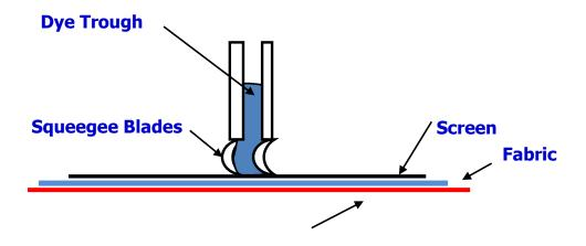
Remember, there is one screen for each color in the pattern. The screens are raised, the blanket precisely moves the fabric to the next color, and the process is repeated. Once each color has been applied, the fabric is removed from the blanket and then processed through the required fixation process. The rubber
