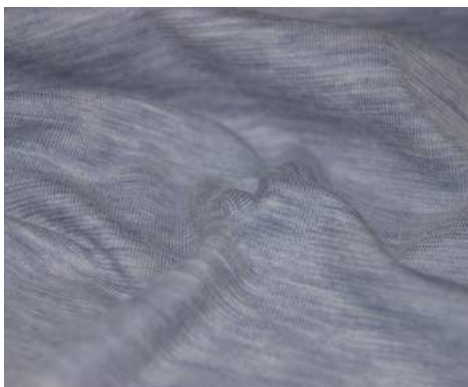
Project: SK-1831-2 Content: 100% Cotton Construction: Jersey
