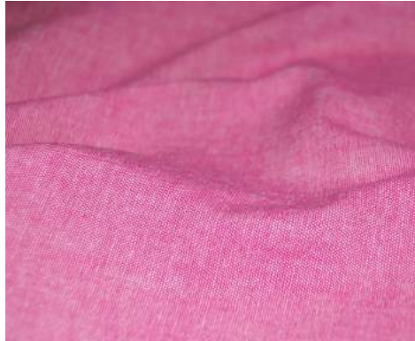
Project: 6174 Content: 100% Cotton Construction: Plain
