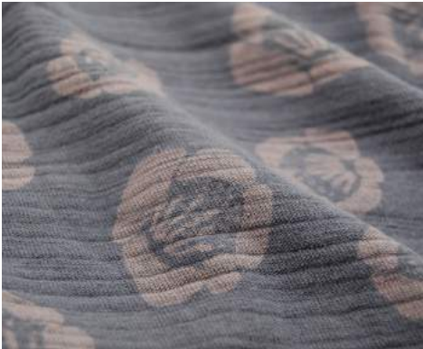
Project: SK-2016-4 Content: 100% Cotton Construction: Jersey
