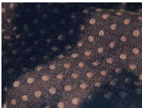
Project: DK-2776-5B Content: 78% Cotton/22% Nylon Construction: Jacquard Comments: Spray bleached
