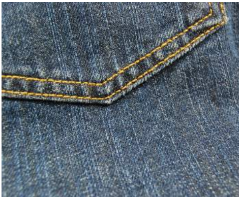
Project: 7068 Content: 100% Cotton Construction: Twill – 3/1 Right Hand
