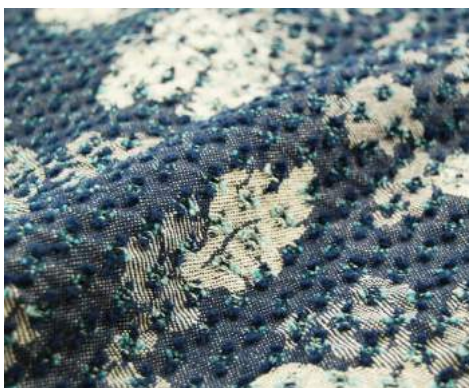
Project: 7018 A Content: 100% Cotton Construction: Jacquard
