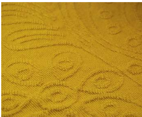
Project: 7011 Content: 100% Cotton Construction: Twill – 3/1 Left Hand
