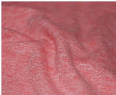
Project: SK-1800-1A Content: 100% Cotton Construction: Jersey
