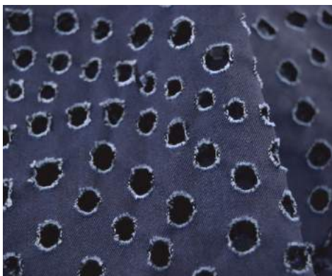
Project: 7020 Content: 100% Cotton Construction: Twill – 2/1 Right Hand
