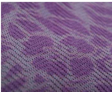
Project: DK-2753-4L Content: 100% Cotton Construction: Jacquard
