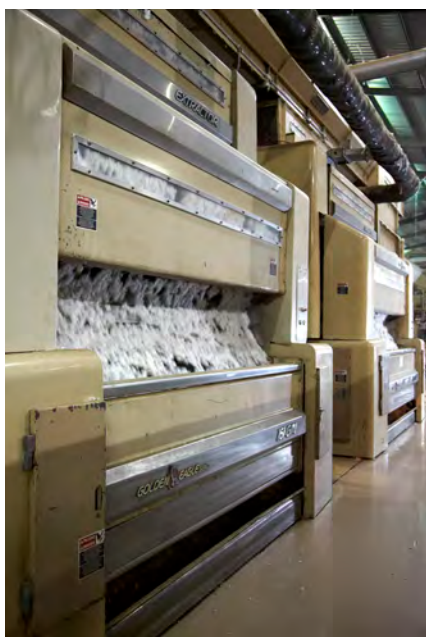
The gin stand separates the cotton fibers from the seed.
