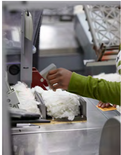
The color of cotton is graded by the high volume instrument.
