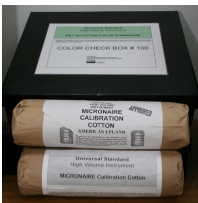
Examples of Universal Color Standards and Micronaire Standards for high volume instrument calibration.
