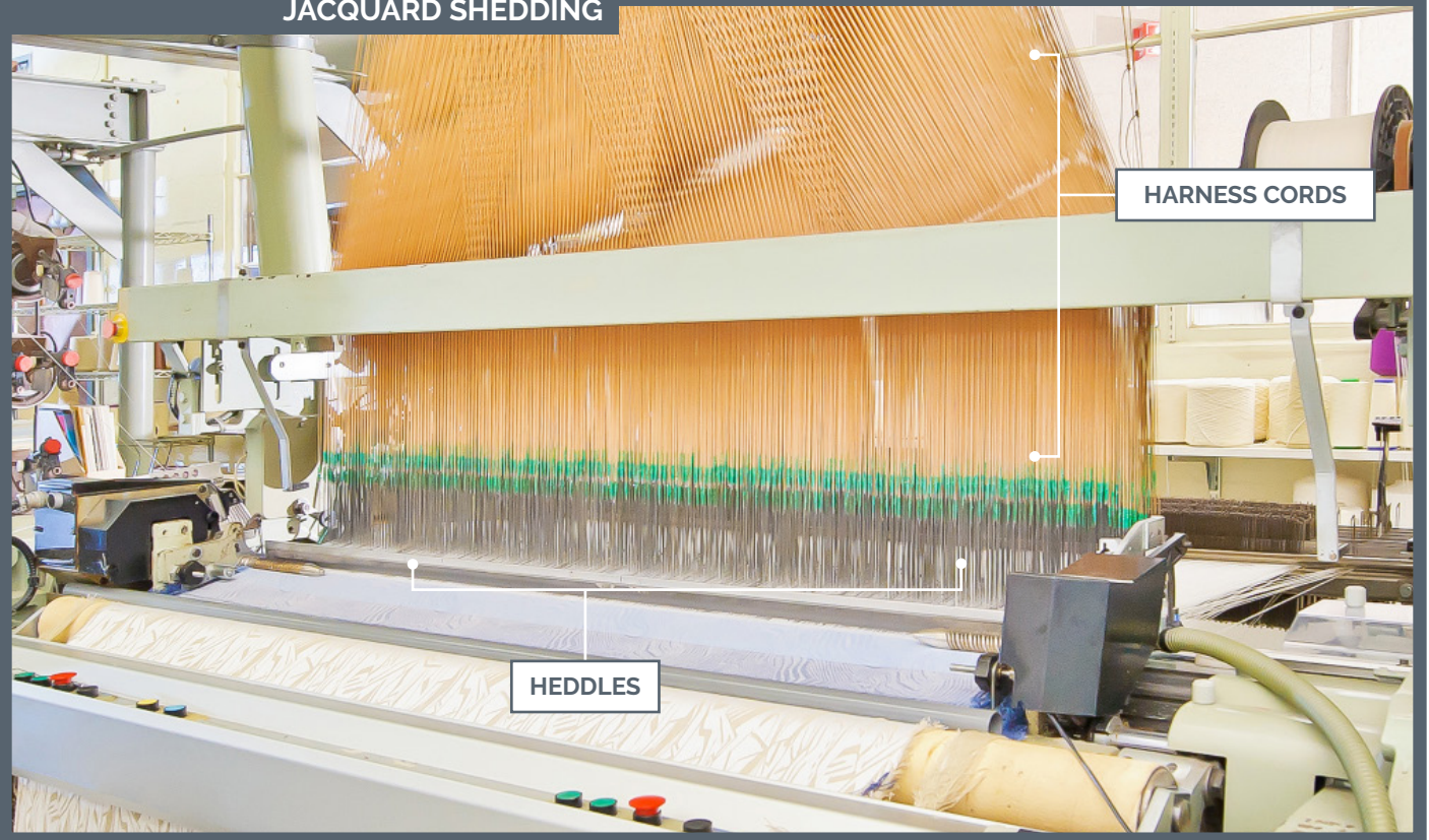
Jacquard loom weaving fabric with a large-scale pattern.
